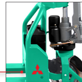
Maintenance free brushless (AC) wheel hub motor
